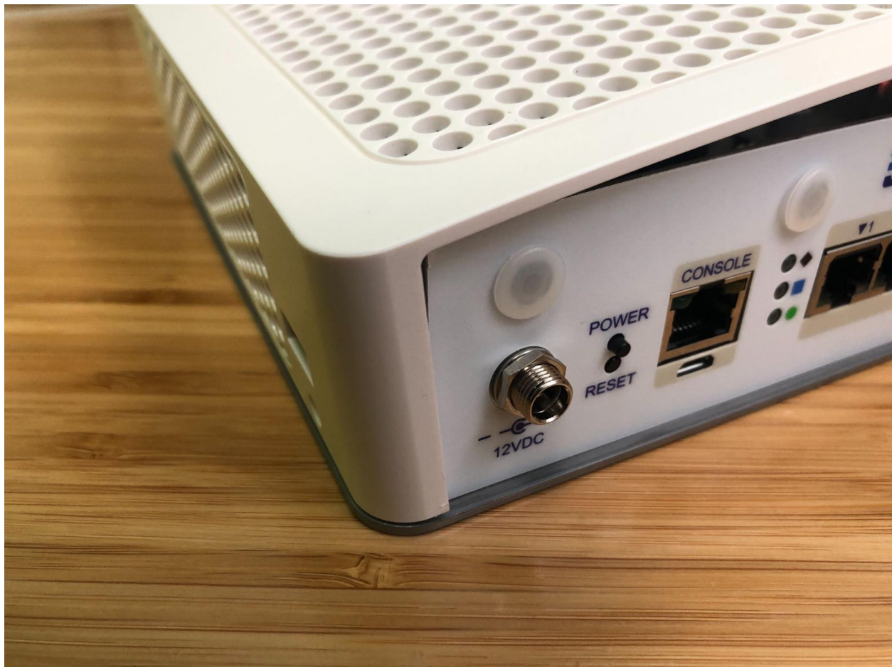
Fig. 50: Aligning the left edge of the lid with the I/O panel
