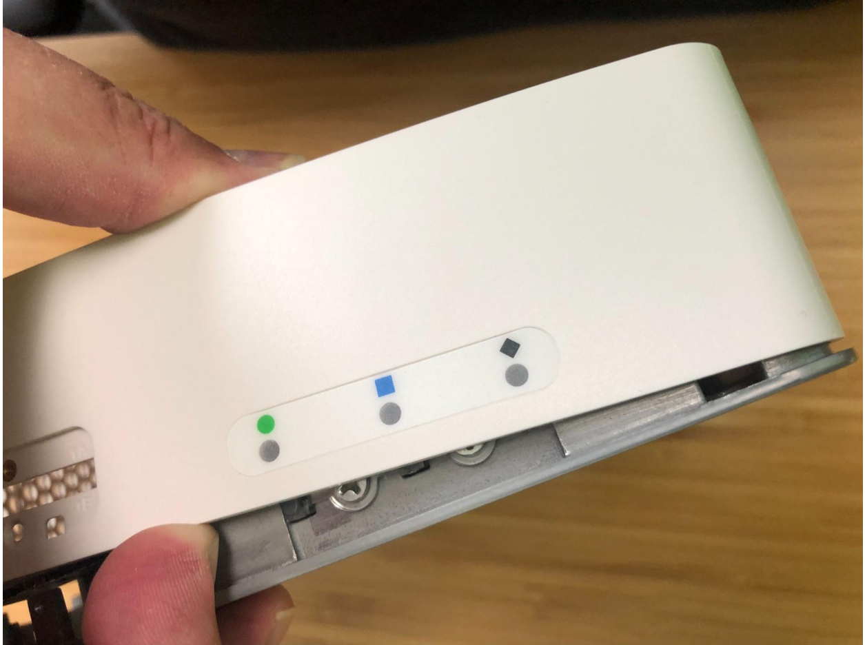
Fig. 52: Replacing the front part of the lid over the LED guides
