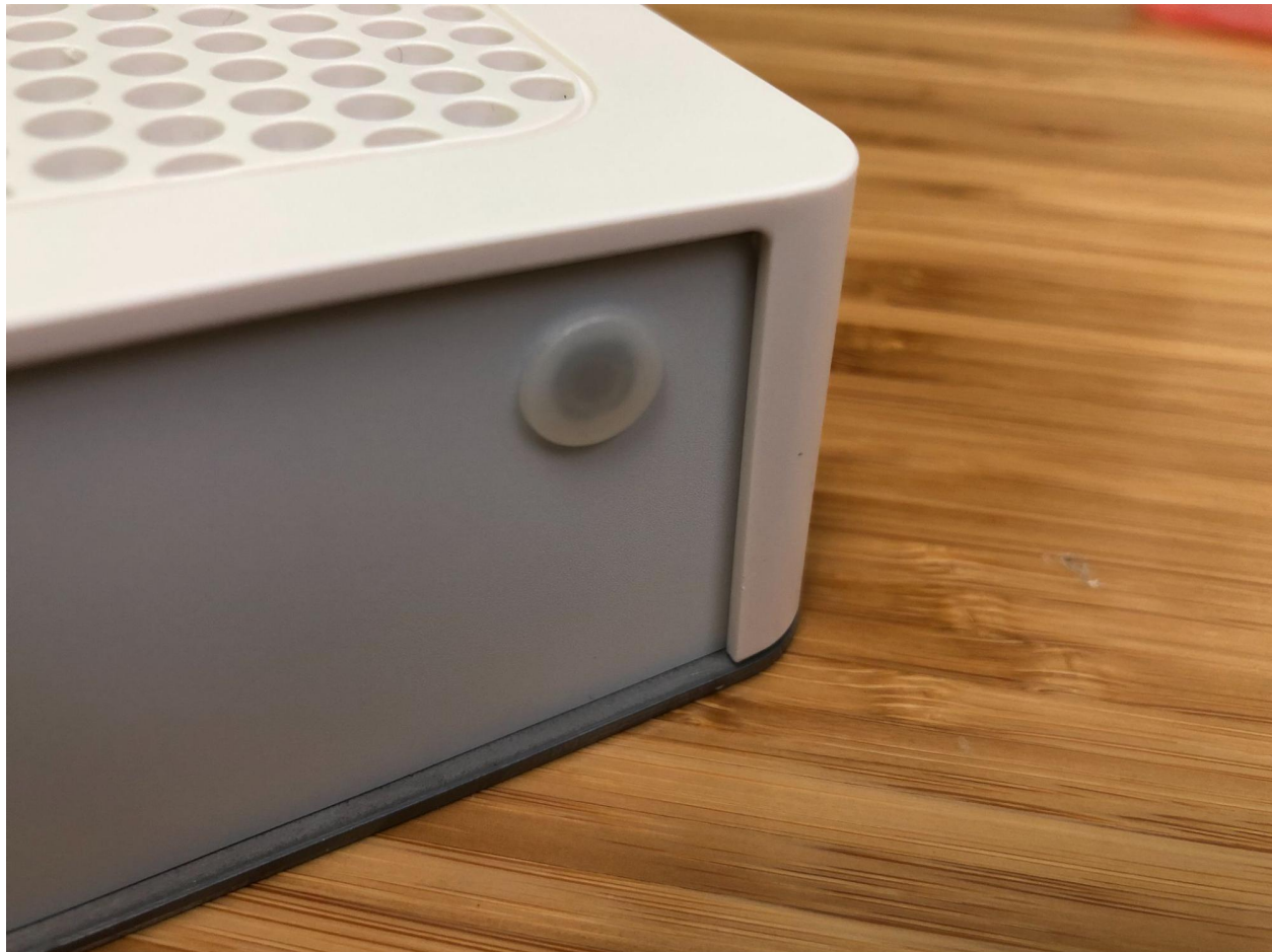
Fig. 5: One of the antenna mounting holes on the I/O panel with its dust cover
