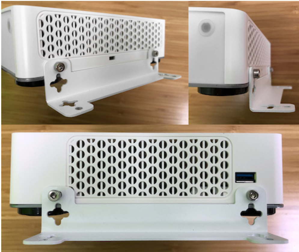
Fig. 7: The Netgate 4200 Outboard Wall Mount Orientation
