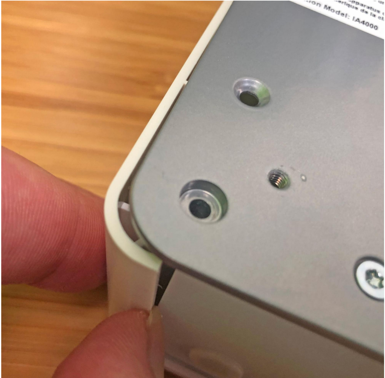
Fig. 44: Lid removal starting at a corner
