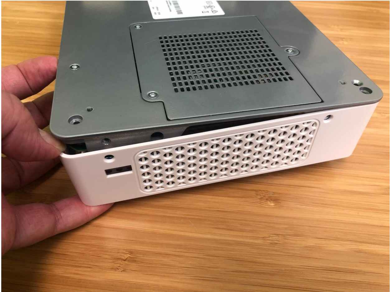
Fig. 45: Separating the lid from the metal base
