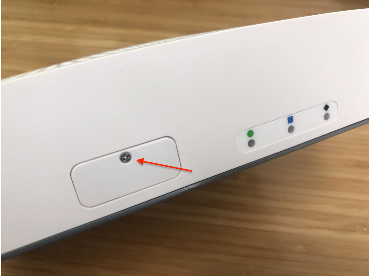
Fig. 39: SIM card slot cover screw location
