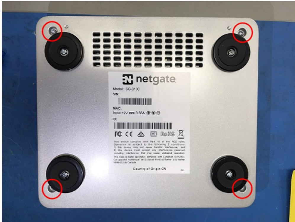
Fig. 4: Removing the SG-3100 Case Screws
