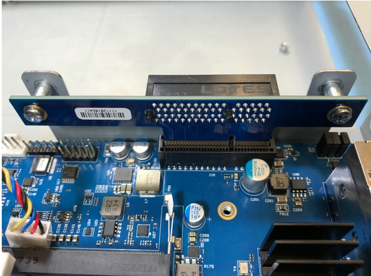
Fig. 25: Align the Riser to the Connector and Insert
