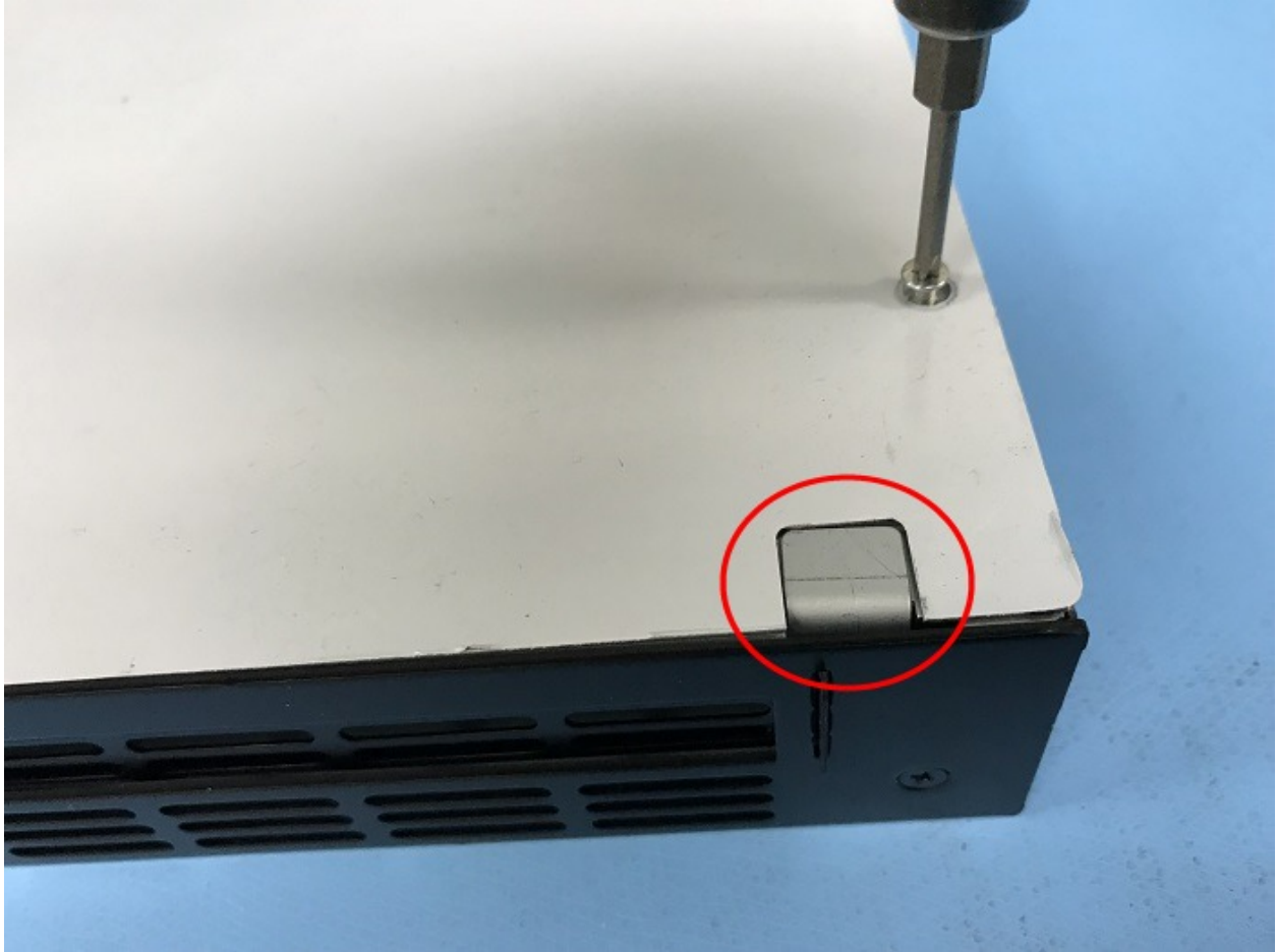
Fig. 17: Proper Placement of the Lid and L-Bracket
