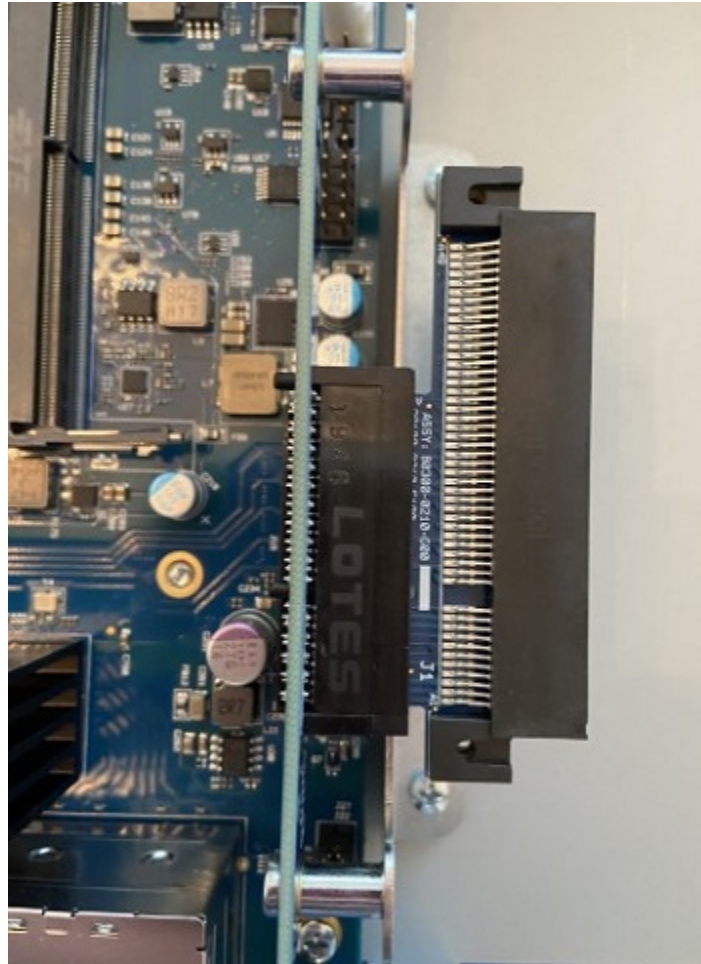
Fig. 28: Extender seated into the Riser
